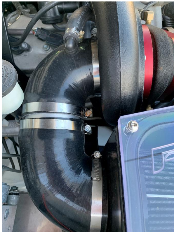
Fitting the air ducting from airbox to the SC inlet – adjust length at the joiner sleeve between the two pieces
